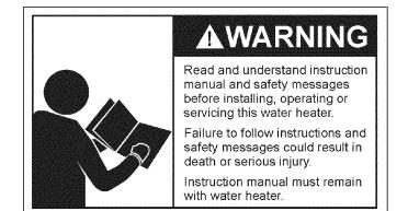
Read this manual first. Then before checking the water heater make sure the electric supply has been turned "OFF", and never turn the electric supply "on" before the tank is completely full of water.
